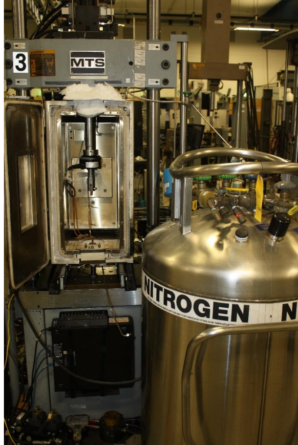
Figure B1. The complete testing setup, including the tensile testing machine and the nitrogen tank used for temperature regulation.
