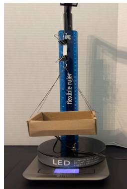
Fig. 2: Apparatus used to measure Young's Modulus of different thicknesses of silicone
