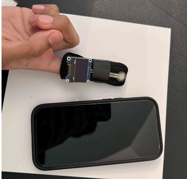
Fig. 17: Proposed fingertip based IOP monitoring device
